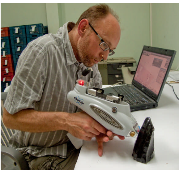
Elemental analysis of a large obsidian blade core from the surface of the West Mound using the Bruker Tracer III V portable X-ray fluorescence [PXRF] spectrometer . Photo Scott Haddow.
