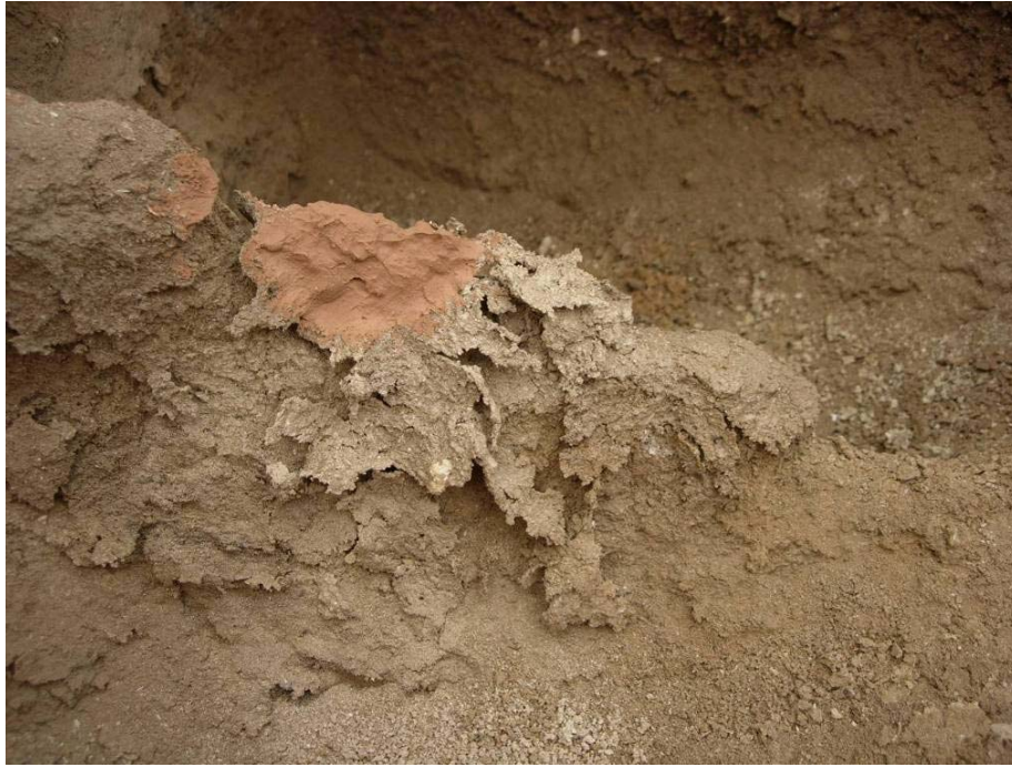
Figure 128: Clay mixed with 25% Primal AC-33 upon drying. Photo Graeme McArthur
