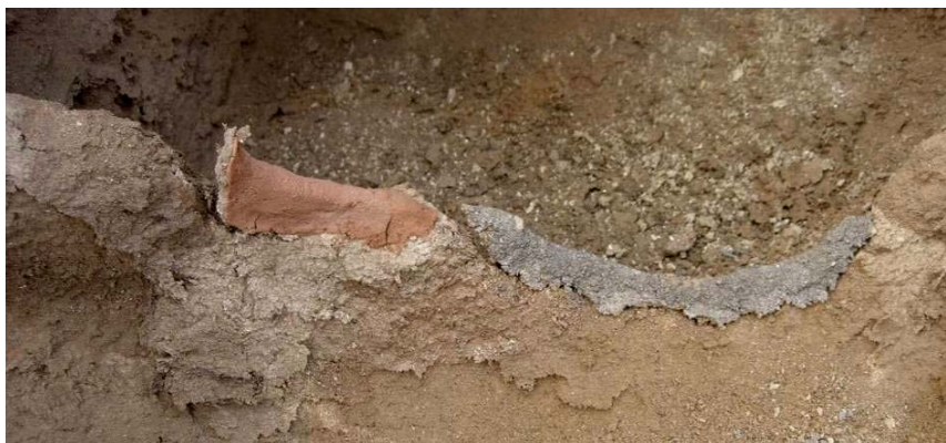
Figure 130: Clay mixture with 50% Primal AC-33 and mortar after drying. Photo Graeme McArthur
