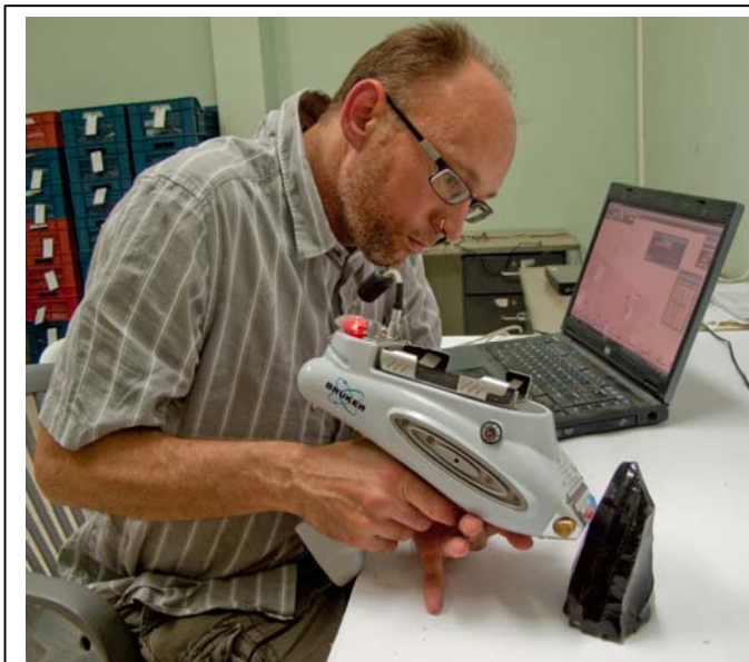
Figure 111: Elemental analysis of a large obsidian blade core from the surface of the West Mound using the Bruker Tracer III V portable X-ray fluorescence [PXRF] spectrometer . Photo Scott Haddow.
